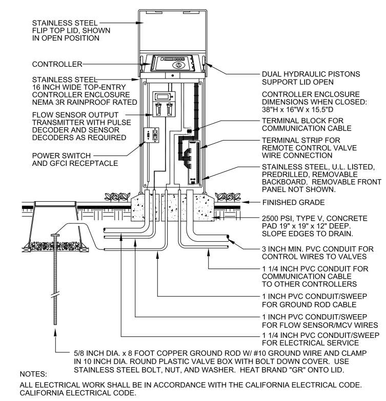
CONTROLLER, ENCLOSURE, AND ALL OF THE REQUIRED COMPONENTS SHALL BE PART OF A PRE-ASSEMBLED SATELLITE ASSEMBLY.
