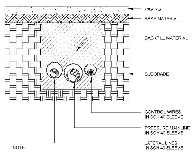
ALL PIPING TO BE INSTALLED IN ACCORDANCE WITH MANUFACTURERS' INSTALLATION SPECIFICATIONS.
