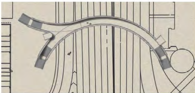
Figure 2.6a Plan view of Concept 2, the concrete arch/girder hybrid option.
