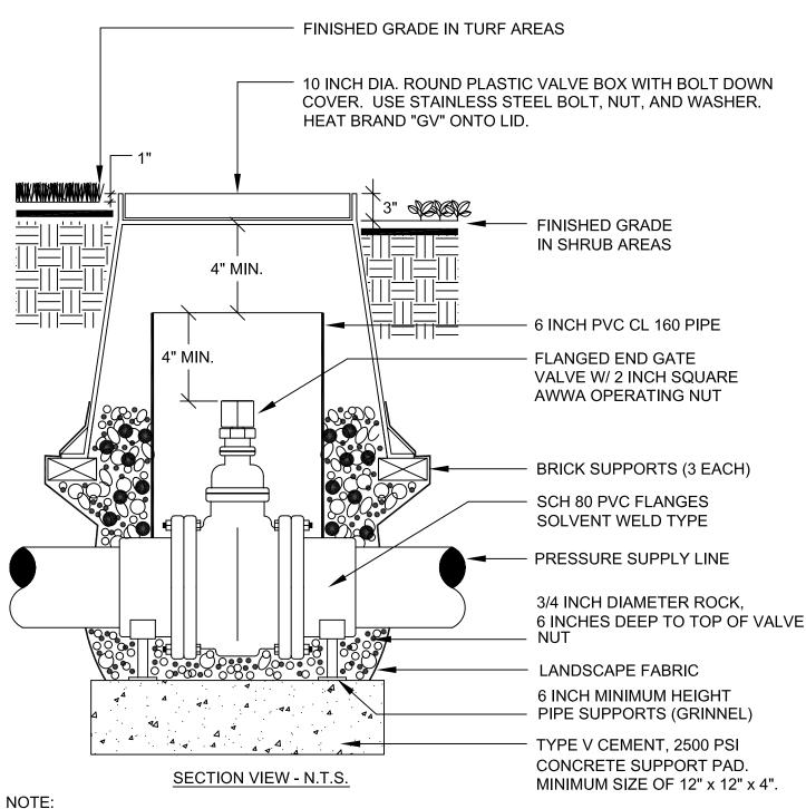
CONTRACTOR TO PROVIDE ONE 5 FOOT LONG TEE WRENCH WITH SQUARE NUT ADAPTER FOR THE OPERATION OF GATE VALVES.
